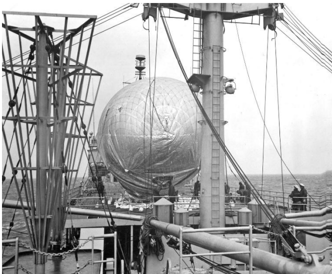
Captive Balloon Supports 'Voice of America' Antenna aboard CGC Courier , 1952 - U.S. Coast Guard, Public domain
